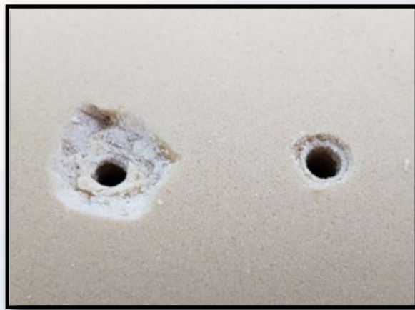
Left: Bone loss after screw removal via chisel/pliers combo
